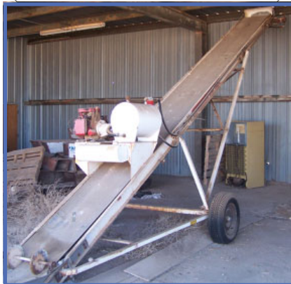
Tyler Conveyer Belt - gas
